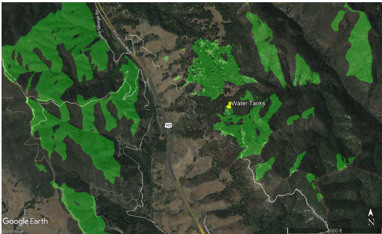
Figure 5 – Line-of-Site Viewshed Analysis for Proposed Water Tanks (The Water Tanks Are Visible to the Areas Shown in Green)
