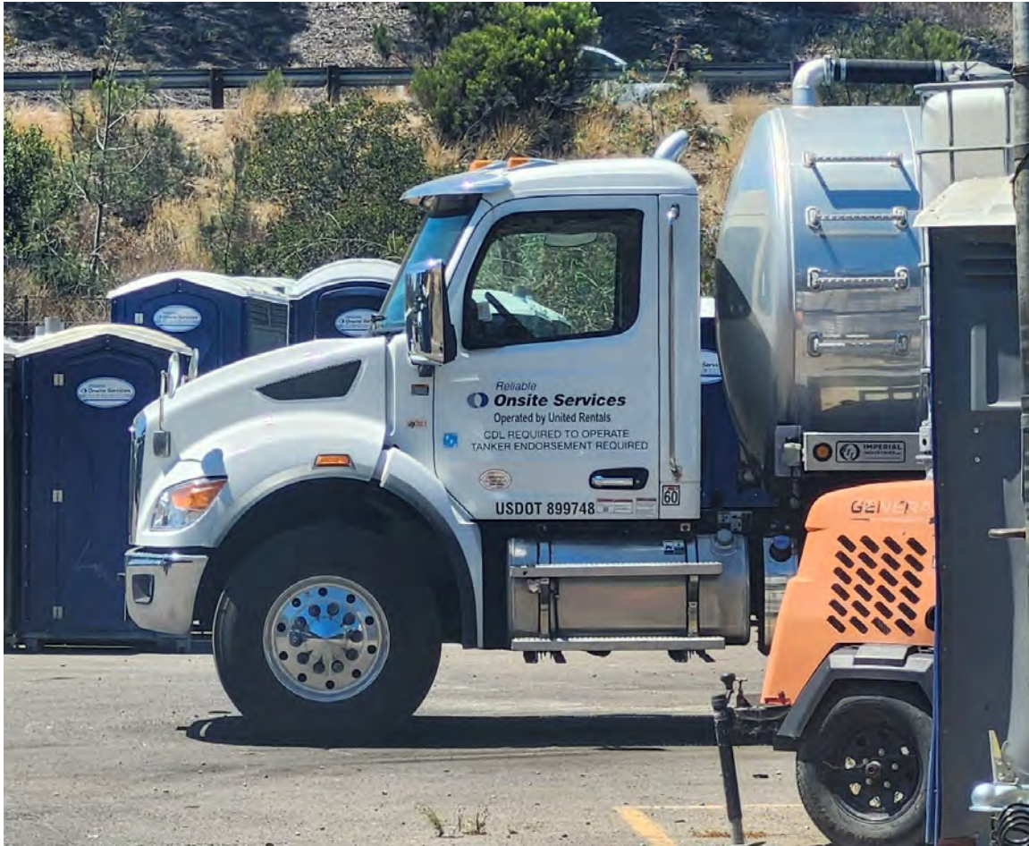
FIGURE 4. Cab-door identification on one of the vacuum trucks — a Peterbilt carrying a stainless Imperial Industries vacuum tank: “Reliable Onsite Services — Operated by United Rentals,” “CDL Required to Operate / Tanker Endorsement Required,” USDOT 899748. That number is United Rentals’ motor-carrier (FMCSA) number — it identifies the company, not the individual vehicle. The 2025 DEHQ permit identifies its 15 trucks by DEHQ decal and California license plate (CHART ONE, Attachment 3), neither of which is legible here, so this unit cannot be matched to a specific permit line from the door markings alone. Whether it is one of the 15 trucks on the permit — or a truck not listed on the permit at all — cannot be determined from this photograph. Either way, it is a United Rentals / Reliable Onsite Services vacuum truck at the 6144 Federal FRAC-tank yard rather than at the Pump Station #1 the permit requires. Photographed June 26, 2026 at 2:42 p.m.
