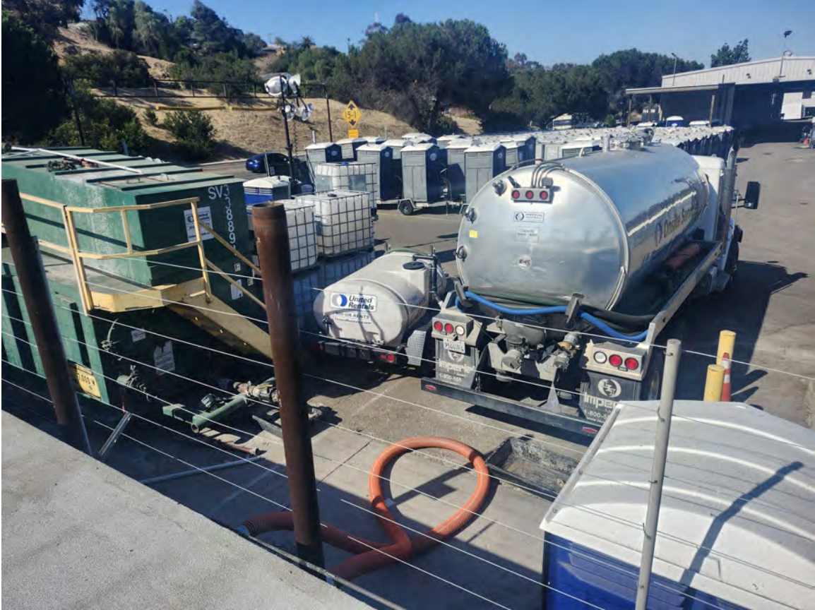
FIGURE 9. The 4,000-gallon “Capacity Waste – 4000” unit (Imperial Industries; California plate 95407F4) parked immediately alongside the FRAC tank on the morning of July 14, 2026. Within the last 7–10 days it can be seen that the 4,000-gallon hauler has been regularly staged adjacent to the FRAC tank. No longer have the smaller vacuum trucks been seen pumping their septage into the FRAC tank. That is significant, because this 4,000-gallon unit is the tank’s outlet — the truck the County says carries the tank’s contents to El Cajon. With no smaller-truck input to the tank, there is nothing for this unit to draw and carry to any receiving facility. The scene — the outlet truck staged at a tank the collection trucks are no longer seen to feed — is consistent with an operation adjusting to the review it is now under. Photographed July 14, 2026 at 9:01 a.m.
