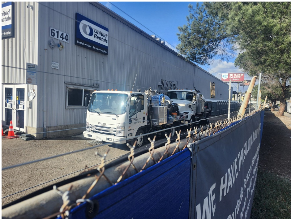
May 27, 2026, shows some of our fleet of 11 2CV trucks that would go into the field and collect poop from our porta-potty rentals. From there they would bring it back to our yard where it would be discharged into Mr. FRAC tank.
