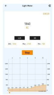
1 foot-candle equals 10.76 lux. The conversion from 1,840 fc to lux = 19,805 lux. The IES design recommendations for parking lots is 30 lux with no more than a 20:1 maximum to minimum variation in light levels. The light levels being generated by Originals (1,840 fc) is 6,000% above the IES recommended maximum level (30 fc) and should not be contributing to the light levels in the adjacent, Big K parking lot. How DSD approved this design is a mystery.
